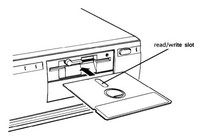
Slide the diskette into the slot until it is in all the way. Then turn the latch down to lock it in a vertical position. This keeps the diskette in place and enables the read/write heads in the drive to access the diskette.
